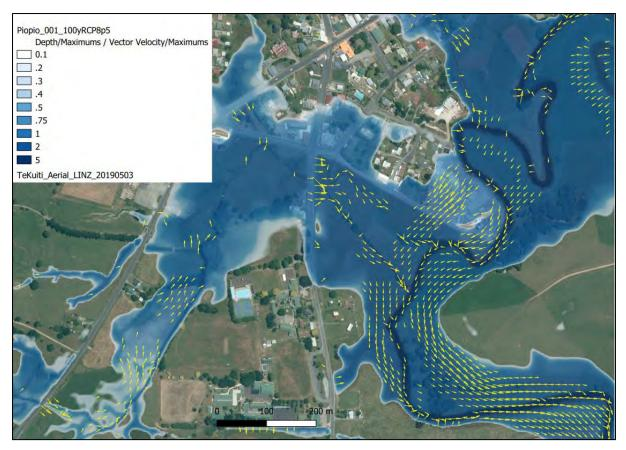
Figure 5.1: Sample maximum flood depth output
